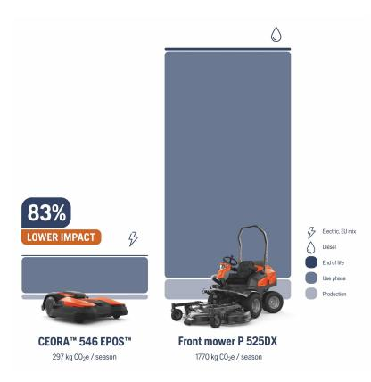
The comparison is made on a scenario of a 30-week cutting season per year. The Lifecycle assessment (LCA) is based on the functional unit of cutting two football pitches (16,000 sqm) of average pitch grass lawn. CEORA is powered by EU electricity grid mix and Husqvarna P 525DX is powered by standard diesel. Result in global warming potential per season (kg  $CO_2e$ /season)\*.
